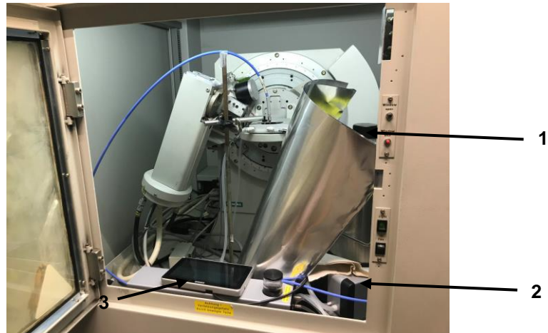
Picture 2: TSL setup with the Dewar (1), water pump (2) and temperature controller (3)
